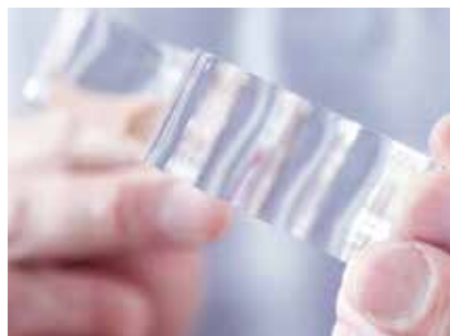
Flame-polished result. Cut up to 40mm acrylic.
